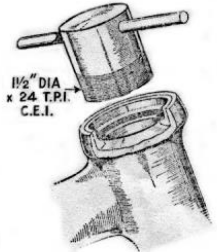
Fig. 42. Steering head ballrace extractor.
